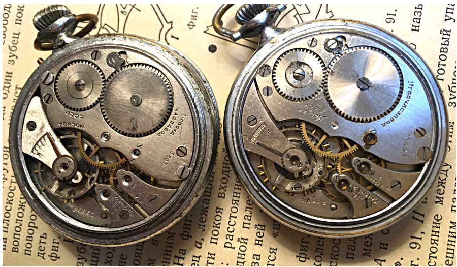
Top & bottom left with a 'Pin Set' movement. (pin between 12 and 1) Top & bottom right very early watch probably with Hampden parts.
